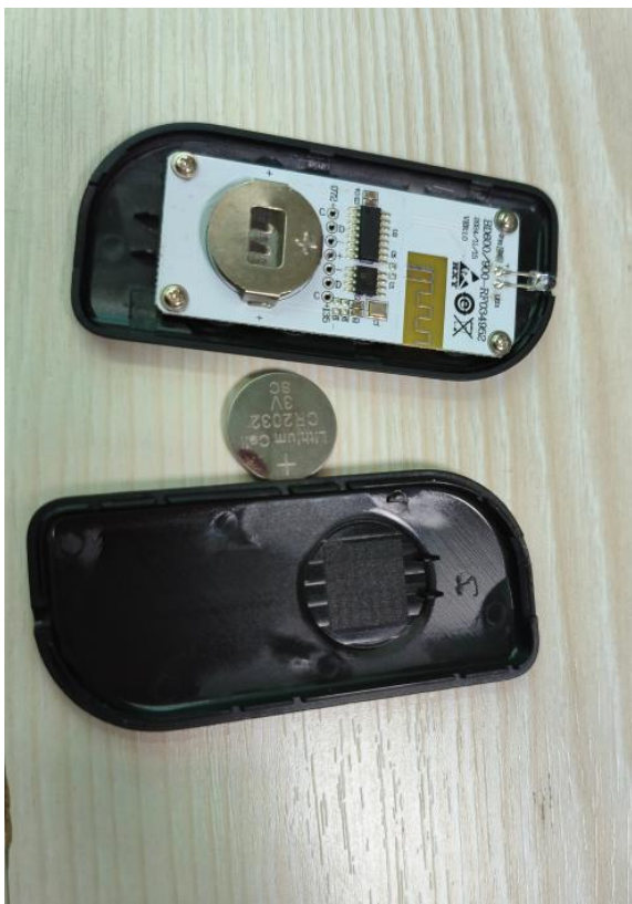
Inner view of remote, battery
